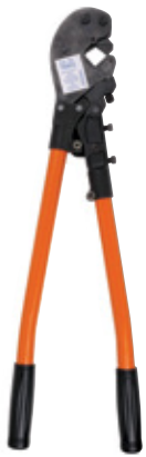
TBM65 Hand-operated crimping tool features Shure Stake mechanism to help ensure a completed crimp. For connectors up to 500 kcmil Cu, 350 kcmil Al.
